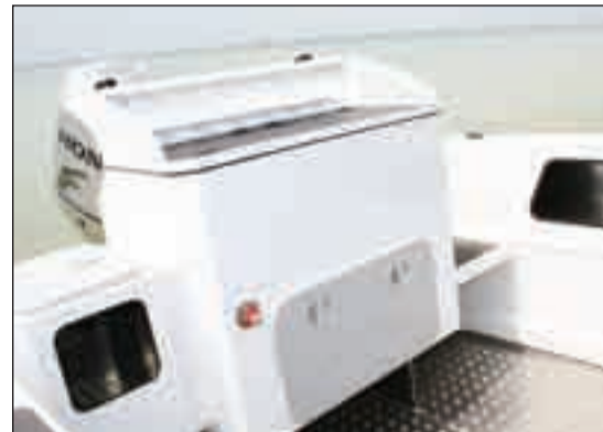
Live bait tank and bait board. Batteries are off the deck in the centre compartment.
