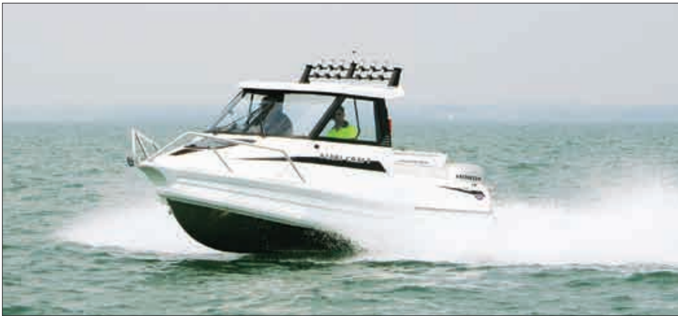
The hull is designed to deflect the water away.
