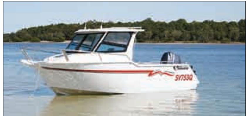
At rest it was very stable due to the reversed chines.
