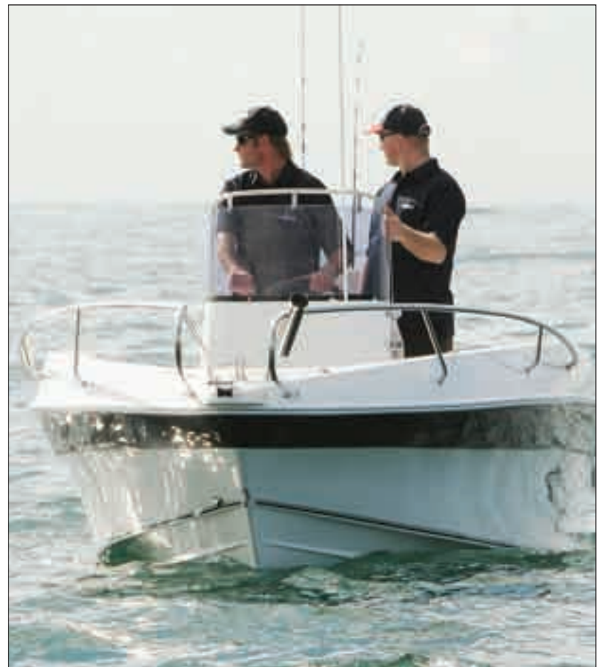
The reverse chine makes this a very stable boat at rest.
