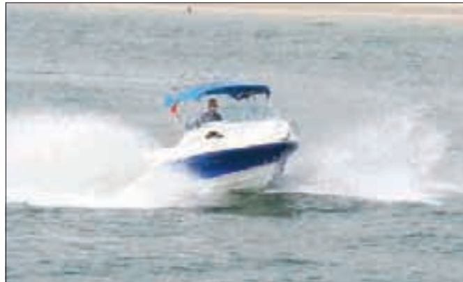
The 21-degree deadrise gives a soft ride when punching through bigger waves.
