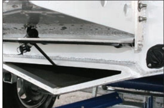
The unique ballast system on Surtees boats gives you a good ride and stability at rest (in open position).
