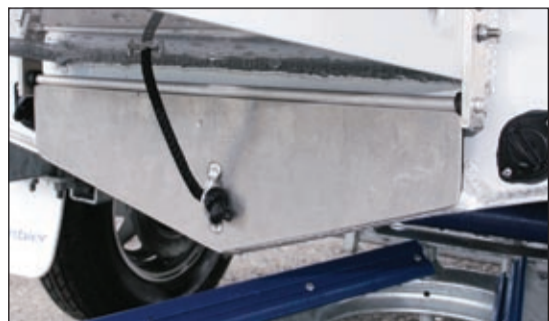
The scupper system for the ballast is operated with a pull cord and spring-loaded cover (in closed position).
