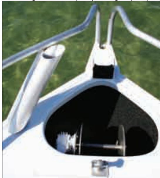
Anchor well with a Stress Free winch fitted.
