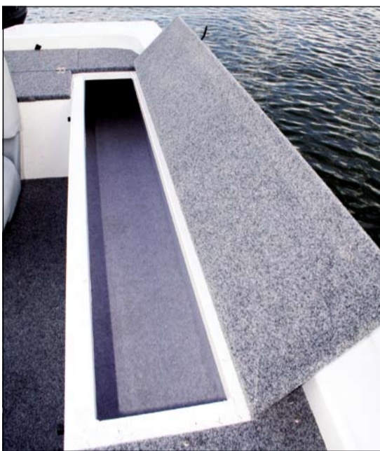
Close-up look at the rod locker.
