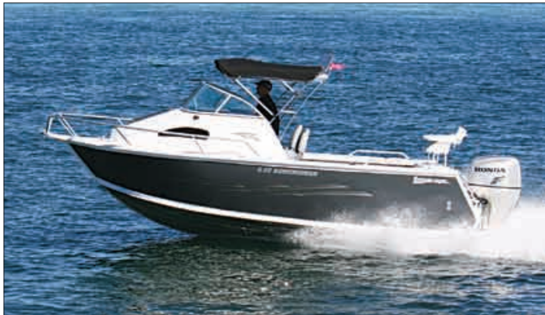
The 135hp Honda 4-stroke has plenty of punch to get the 6m Seascope up and planing.
