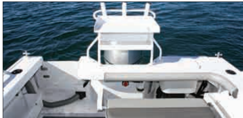
Transom door on the left, folding rear lounge on the right and bait board centre are some of the features that make this boat a good all-round package.
