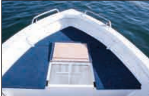
Storage under front casting platform.
