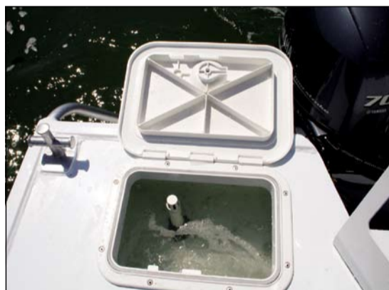
Plumbed live bait tank as standard.
