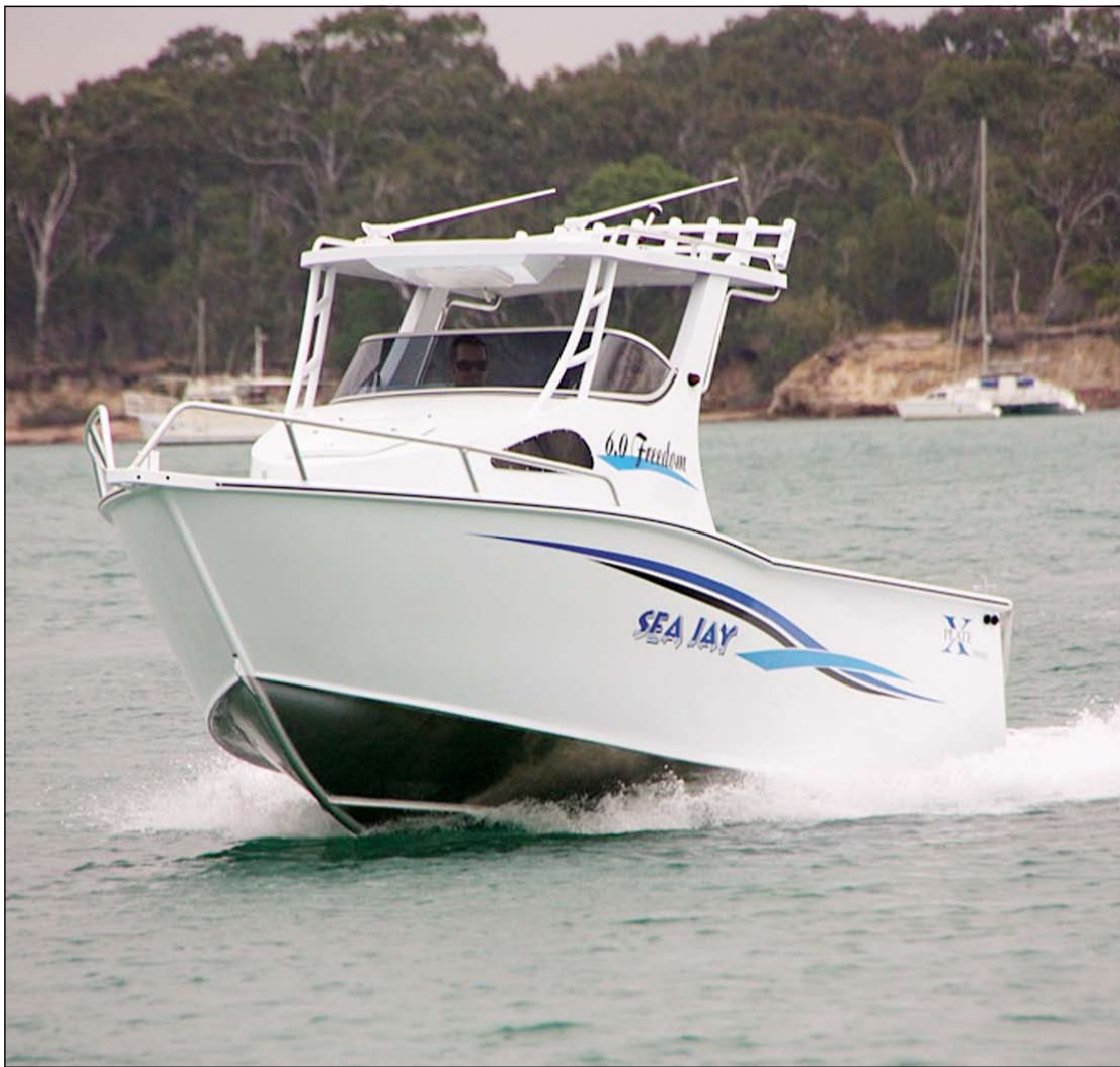
The high swept bow deflects the spray in rough conditions. Photo: Sea Jay
