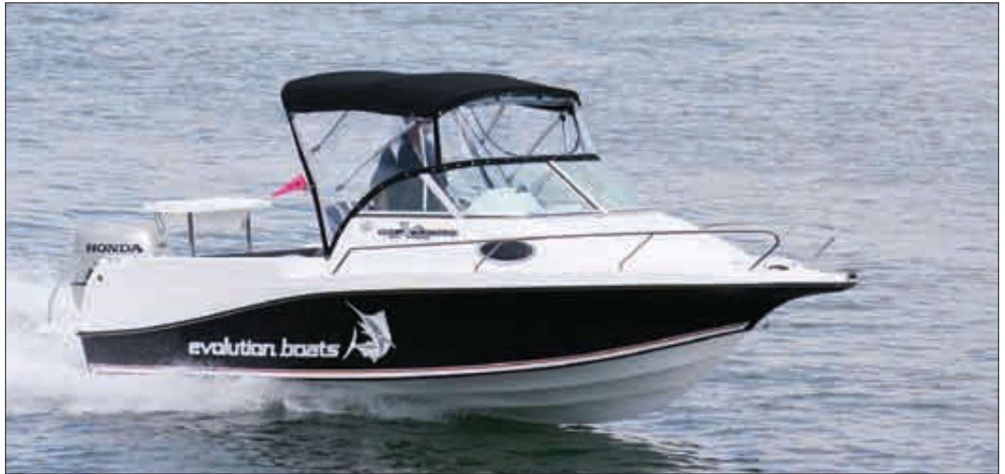
The deep-V and wide transom on the hull gives you a smooth ride and stability at rest.
