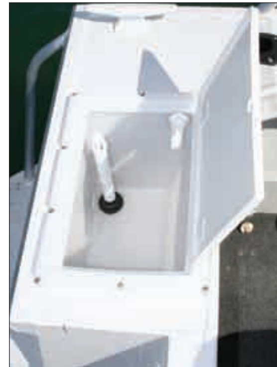
Plumbed live bait tank.
