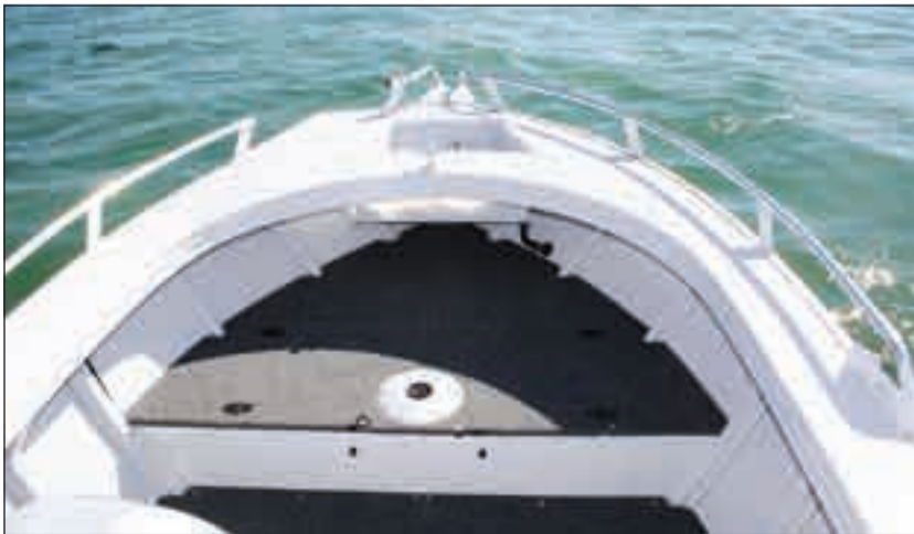
There are two hatches on the front casting platform.
