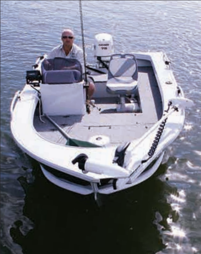
Large front casting platform and wide side decks give you plenty of fishing room. You can also see the optional rod locker fitted on the starboard side of the boat.
