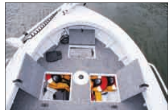
Storage under the front casting platform.
