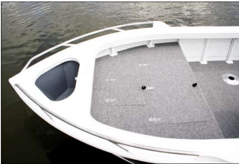
Front casting platform with two storage compartments plus an anchor well.
