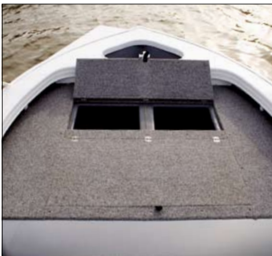
There are two storage compartments and a massive keeper tank under the front casting platform. Note the anchor well and electric motor bracket.
