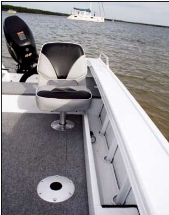
The test boat was fitted with a long side storage pocket. You can option up and have a rod locker fitted.
