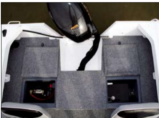
Battery storage and a plumbed live bait tank are located under the rear casting platform.
