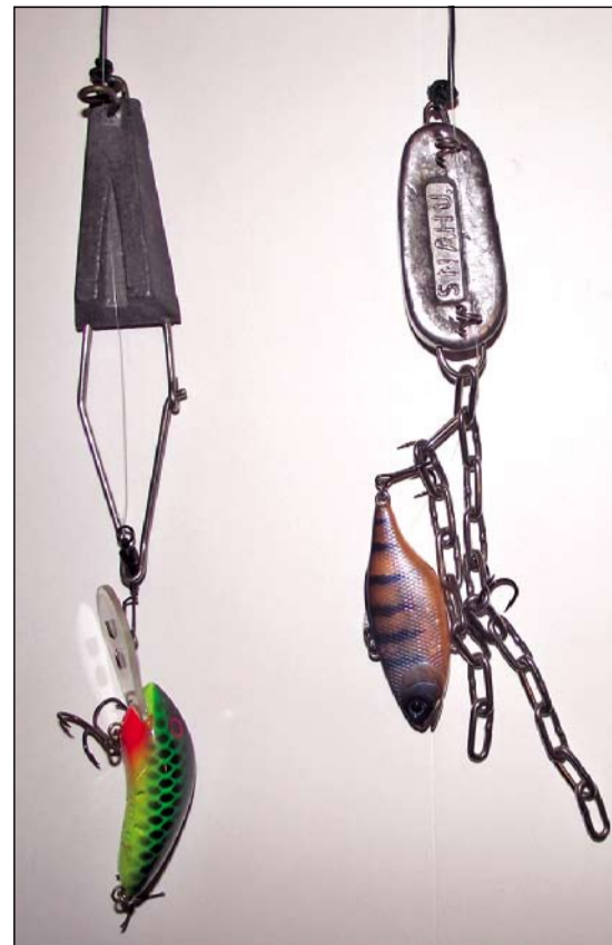
Bomb style lure retrievers (left) and a Tackle Back, Snahu Recover "A" (right).
